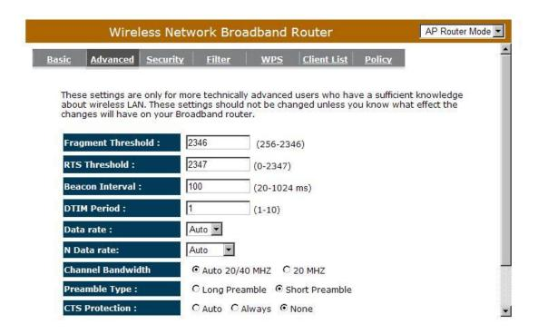
**Fragment Threshold:** This specifies the maximum size of a packet during the fragmentation of data to be transmitted. If you set this value too low, it will result in bad performance.
