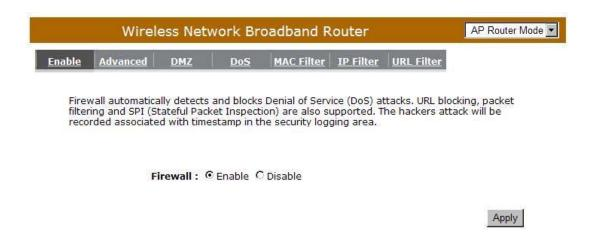
Note: To enable the Firewall settings select Enable and click Apply
