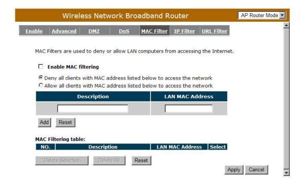
**Enable MAC Filtering:** Check to enable or disable MAC Filtering.
