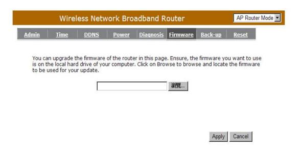
Once you've selected the new firmware file, click **Apply>** at the bottom of the screen to start the upgrade process
