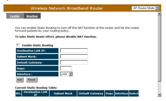
**Destination LAN IP:** Specify the destination LAN IP address of static routing rule.
