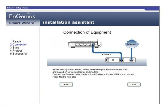
Check the MODEM and ESR-9753 connection. It should be as shown below.
