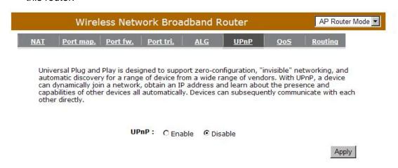
Enable/Disable UPnP: You can enable or Disable the UPnP feature here. After you enable the UPnP feature, all client systems that support UPnP, like Windows XP, can discover this router automatically and access the Internet through this router without having to configure anything. The NAT Traversal function provided by UPnP can let applications that support UPnP connect to the internet without having to configure the virtual server sections.
