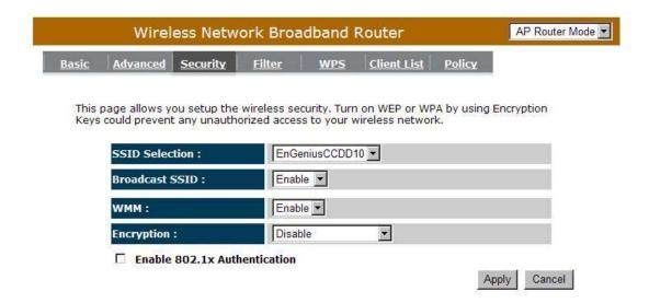
**ESSID Selection:** This broadband router support multiple ESSID, you could select and set up the wanted ESSID.
