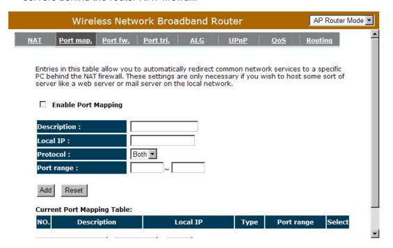
**Enable Port Mapping:** Enable or disable port mapping function.
