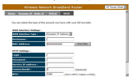
PPTP allows the secure connection over the Internet by simply dialing in a local point provided by your ISP provider. The following screen allows client PCs to establish a normal PPTP session and provides hassle-free configuration of the PPTP client on each client PC.
