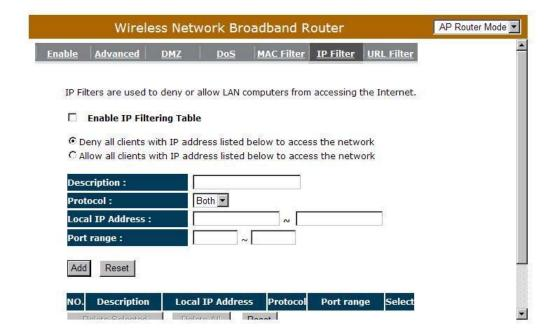
Enable IP Filtering: Check to enable or uncheck to disable IP Filtering.
