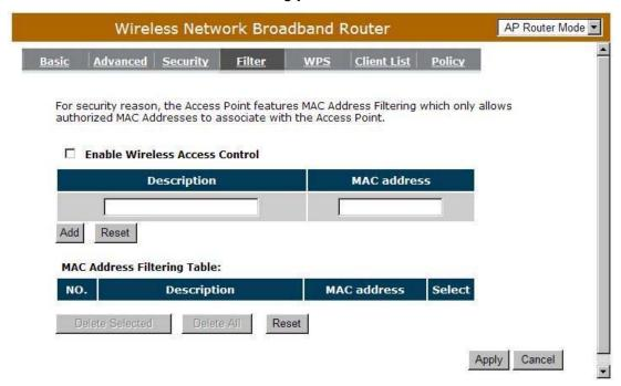
Enable wireless access control: Enable the wireless access control function
