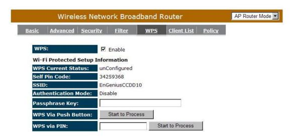
**WPS:** Check the box to enable WPS function and uncheck it to disable the WPS function.
